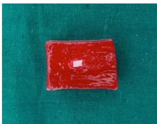
Figure 2. Readings Obtained on Enamel Block using Vickers Micro-indenter
